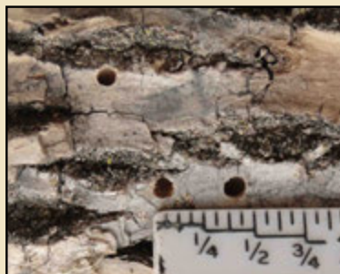
Exit holes: Typically round and variable in size (1/8 inch or more).
