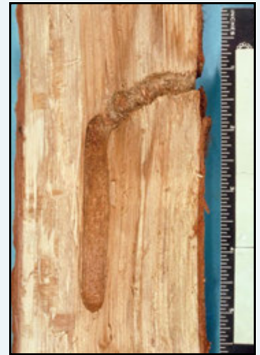
Tunnels: Large, 1/2 inch wide. Extend deep into the wood. 10
