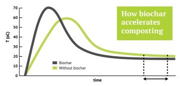
Biochar increases the temperature in the compost process, accelerating material decomposition
