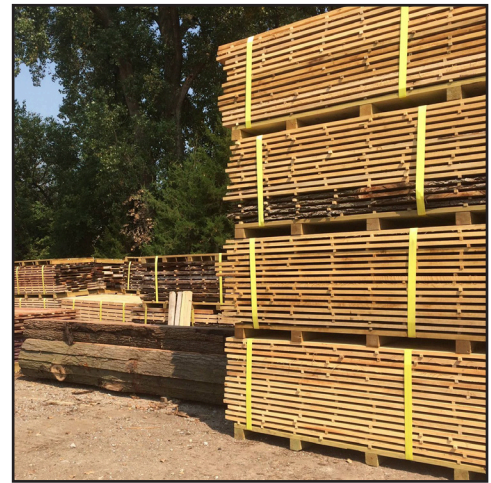
Stickered lumber prepared for kiln drying at Big Red Sawmill in Palmyra, NE
