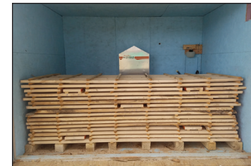
Dehumidification kiln drying rough lumber.
