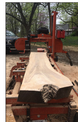
Slabs of wood going through portable sawmill. Slab residue can be used as compost or mulch.
