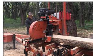
Portable sawmill cutting rough lumber.
